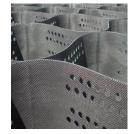
EnviroGrid® EGA 40 sections are manufactured from 58 strips of HDPE, resulting in a section length of 29 cells. Each strip is the approved width and 142 inches (3.6m) in length.
